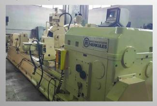
Having extensive experience and an active network in this industry, CNC Design Thailand had identified a suitable machine in Europe. This was a Herkules WS450, suited for grinding the rolls of POSCO-Thainox. The roll grinder was shipped to our Thailand factory in Bangkok and the work began.
